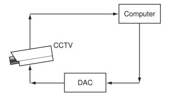
The digital CCTV camera is connected to a computer. The computer can make the camera move in any direction by sending out digital signals. The computer system has a 400 gigabyte hard disk.
